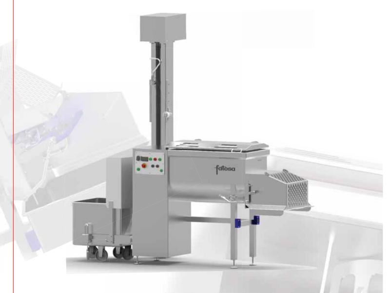
The mixer A300 DL is equipped with one arm with T-shaped paddles easily removable that ensures a comfortable and perfect cleaning. The A300 DL standard model is equipped with 1 mixing speed and two turning senses, although optionally the machine can be supplied with adjustable Variable Speed by means of a digital potentiometer which ensures an ideal mixing for different types of product.
