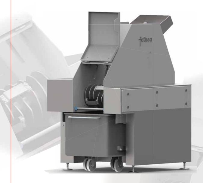
The Flaker of frozen blocks CBC LP2 is a machine designed to cut frozen blocks of meat or other products at temperatures of up to -20  $^{\circ}$ C. Thanks to the rotation of a drum equipped with 4 U-shaped blades, this equipment allows to reduce the size of the blocks to irregular portions to facilitate the later processing in bowl cutters or grinders. The machine is equipped with a 7.5 kW motor and can reach an output of up to 2,000 Kg / h.
